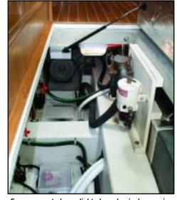
Easy access to large, lighted mechanical space in main cabin, through a hinged hatch with gas cylinder lifting assists. Ample space for generator and water maker has been included.
