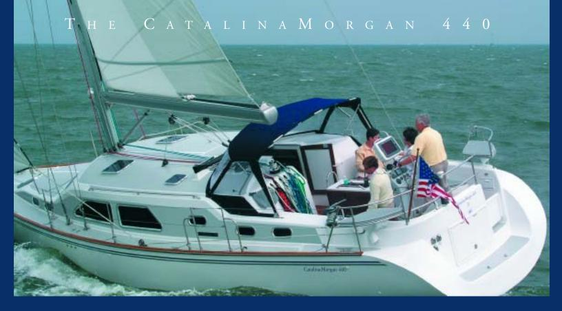
Built-in Catalina quality means thirty-one inch lifelines on removable tapered stanchions that make going forward safe and secure. Stern gates that retract into stern rails, and won't rattle underway. A solid teak cap rail with chafe guards for dock lines. An extruded aluminum cap rail is also available.
