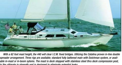
spreader arrangement. Three rigs are available; standard fully battened main with Dutchman system, or available in-mast or in-boom sytems. The mast is deck stepped with stainless steel thru deck compression post, is the ultimate in strength and is designed to eliminate potential leaks.
