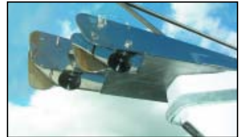
Stainless steel offset double anchor rollers standard.
