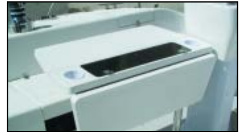
Fiberglass cockpit table with foot brace. Teak leaves and bin lid are available.
