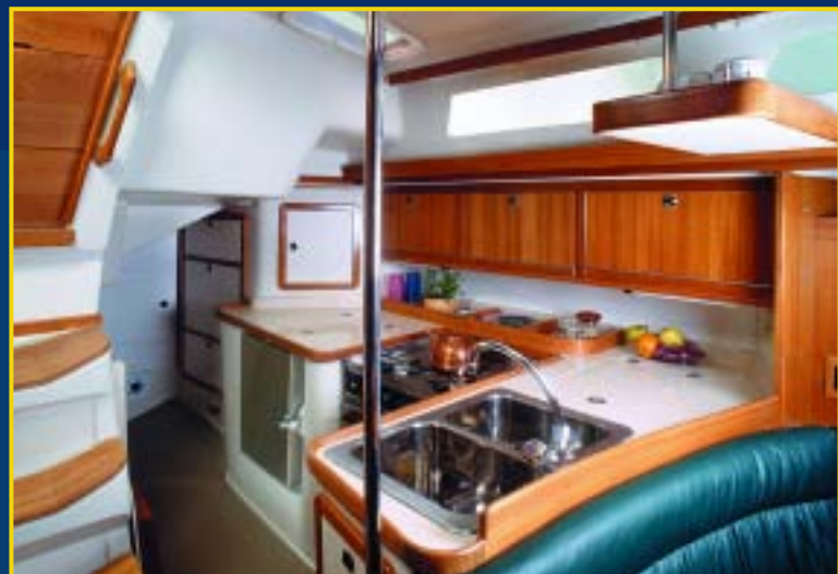
The two cabin galley has 10 cabinets, plus dry storage food storage locker. Top and side loading icebox provides accessible food and beverage storage.
