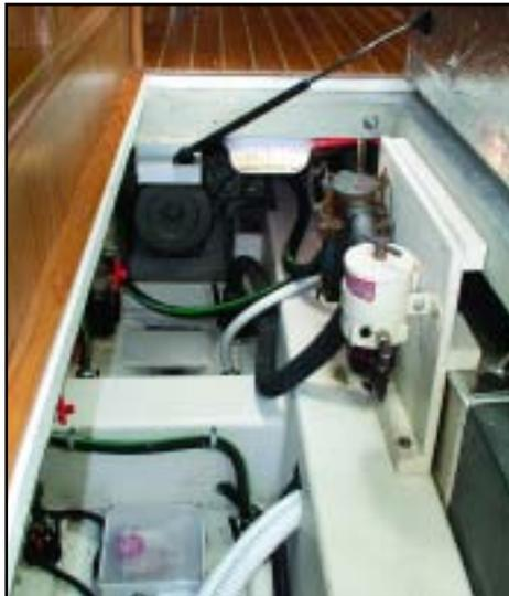
Easy access to large, lighted mechanical space in main cabin, through a hinged hatch with gas cylinder lifting assists. Ample space for generator and water maker has been included.
