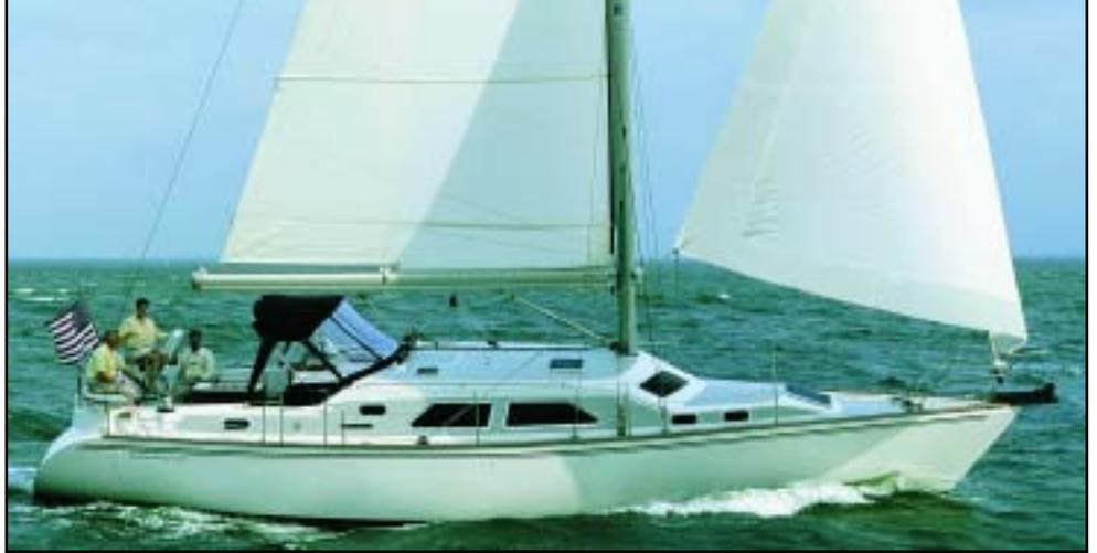
With a 62 foot mast height, the 440 will clear I.C.W. fixed bridges. Utilizing the Catalina proven in-line double spreader arrangement. Three rigs are available; standard fully battened main with Dutchman system, or available in-mast or in-boom systems. The mast is deck stepped with stainless steel thru deck compression post, is the ultimate in strength and is designed to eliminate potential leaks.
